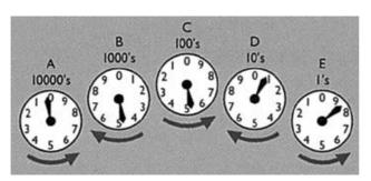
A reading on this example meter is taken by reading the dials from left to right, (A to E). The direction that each dial travels is shown. This reading is **04508**.To check your average daily consumption, take readings at the same time of the day, several days apart.
